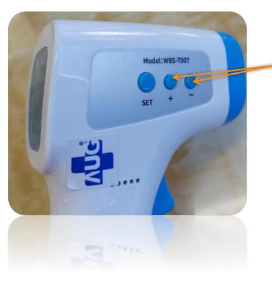
Press the ""+" & "-" in order to adjust the setting to the desired value according to the deviation.
