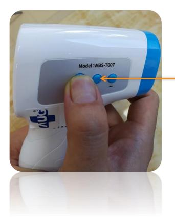
Press the "Set button" for about 3 seconds. After you release the button, the screen will be as showed.
