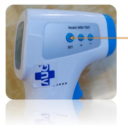
Finally press the "Set button" two (2) times to complete the set up.
